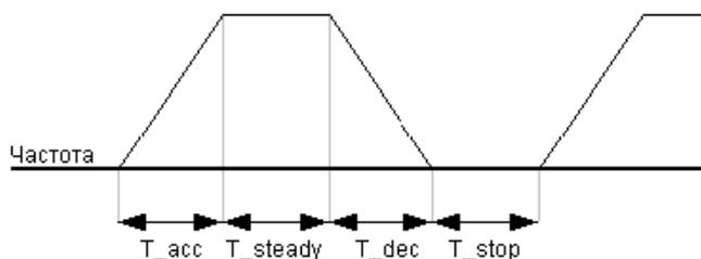
$$\text{Пример 2) } H76 = \frac{T_{dec}}{T_{dec} + T_{steady1} + T_{acc} + T_{steady2}} \times 100[\%]$$
