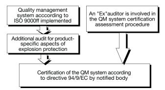
TURCK's manufacturing sites for explosion protected devices are certified according to ISO 9001 and have a quality system approval.
