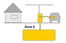
Intrinsically safe devices designed for use in zone 0 must meet category "ia" safety standards and must have no live contacts. Galvanic isolation between intrinsically safe and non-safe devices is to be preferred. If grounding of the intrinsically safe circuit is required for functionality, this must be done outside zone 0, but as close as possible to zone 0. The devices must as well be approved for gas groups IIA, IIB and IIC.
