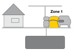
Any device certified for zone 1 must be group IIA, IIB or IIC and at least category "ib".
