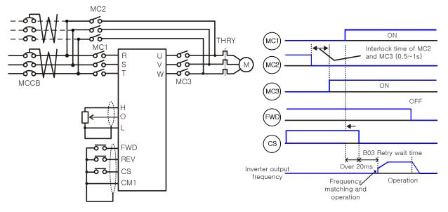
Example) Assigning 12[CS] to an intelligent input terminal [DI2].
