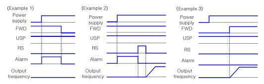
Example) In case Assign 13[USP] to an input terminal (DI2)
