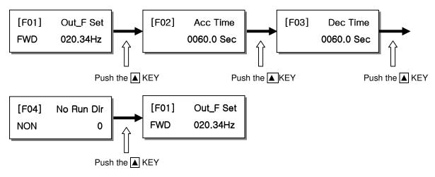
2) Setting method of parameter value (Example: Change of frequency parameter)
