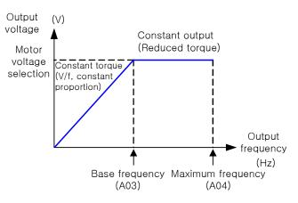
• The base frequency (A03) should be same as the maximum frequecy (A04) for constant torque.
