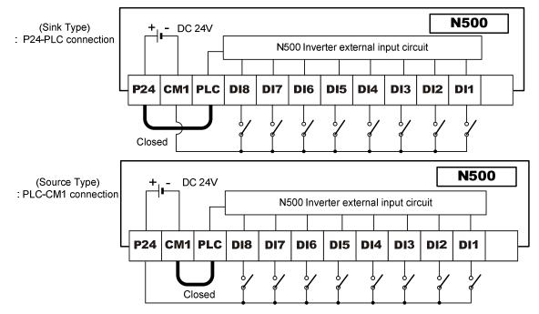
• In case of using the external power source of inverter
