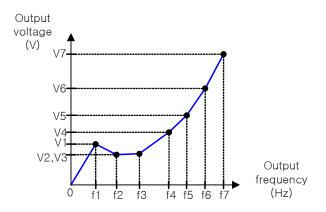
(Note1) Even if you set 800V for free V/f voltage1-7, output of inverter can't be more than the input voltage or the AVR setting voltage.
