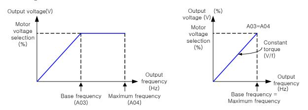
• The base frequency is the nominal frequency of the motor, this value can be found on the nameplate of a motor.
