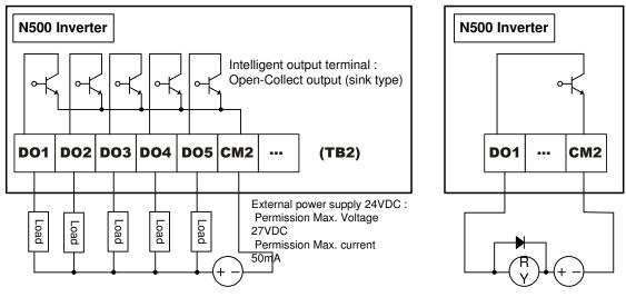
Note) Use Inverter output terminals to operate samall relays when it needs over 50mA.
