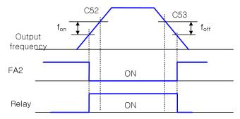
Setting frequency Fon : 1% of Max. Frequency Foff : 2% of Max. Frequency
