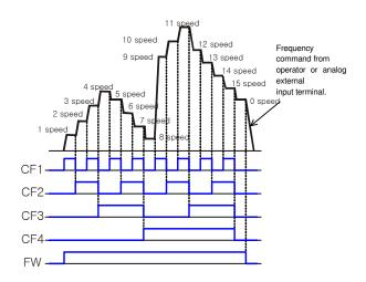
Example) The settig method for Multi-speed operation from control terminals
