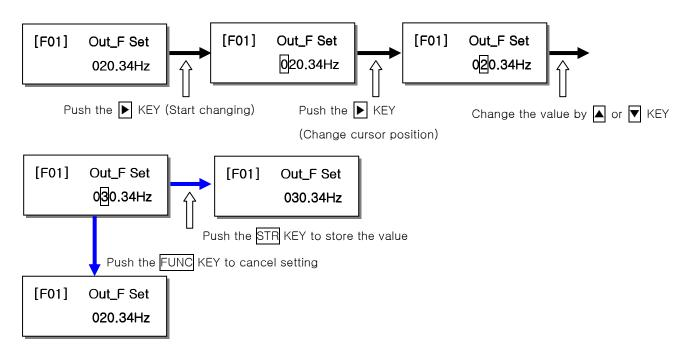
Note) Although pushing the **STR** KEY, the store function will be canceled and the parameter value will be back to the previous value when changing mode which is unchangeable on run and setting value exceed the range..
