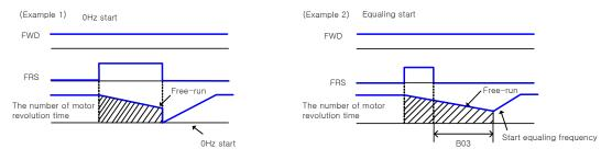
Start 0Hz regardless of the motor speed. On 0Hz start, the retry wait time is disregarded.
